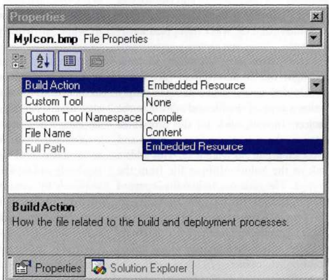
Figure 3 Embed a Resource. When you assign an icon to a custom control, you can set the Build Action on the bitmap file to Embedded Resource. This causes VS.NET to embed the file in the assembly, so you don't need to ship the icon along with the binary file that contains the control.
